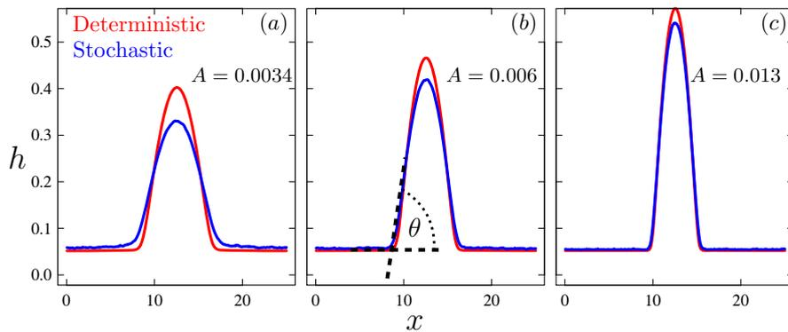
**Fig. 3.** Deterministic and stochastic droplet spreading from numerical simulations of Eq. (10) at the stationary state. The stochastic shapes have been averaged over 100 noise realizations. Panels (a) through (c) correspond to increasing values of  $A$ , as given.
